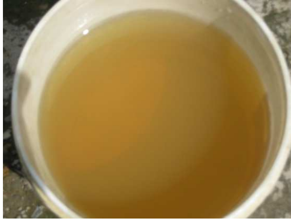
Fig. No. 59:- Sample of Groundwater along drain containing objectionable colour, odour, taste & suspended solids.
